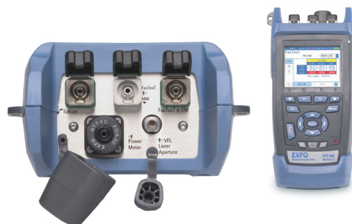
The green ring on the EXFO Universal Base plate indicates that it has an APC ferrule.
